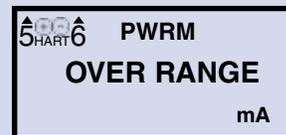
The PIE 311Plus is supplying the loop voltage. There is a control loop error. This may be a transmitter (set for upscale burnout) with a bad or missing sensor, or a short in the loop. The red ERROR LED will also flash.
