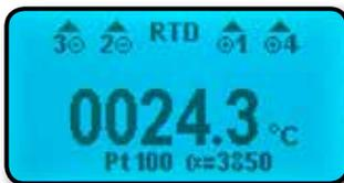
Here is an example where connections are made to a 4 wire sensor and the 311Plus indicates that only Wires 1, 2 & 4 are connected. There may be a loose connection or a break in wire 3 somewhere between the sensor and the 311Plus.
